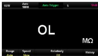
Figure 3-3 Reading of short-circuit test leads
