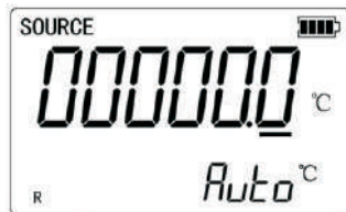
Picture 3.5-1 °C temperature display
