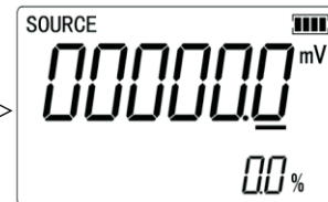
Picture 1.1-6 Voltage output 1000mV
