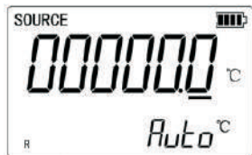
Picture 3.2-1 Auto cold junction temperature compensation
