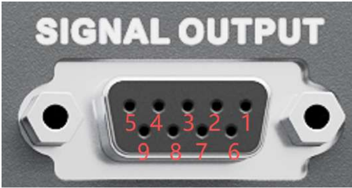
Figure 15-2 Signal Output Interface
