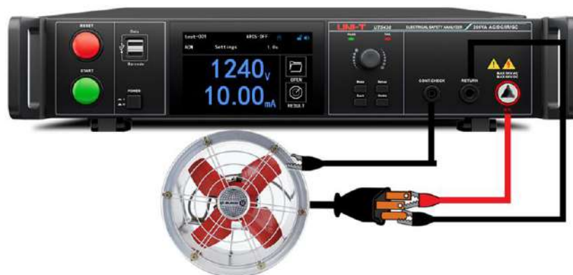
Figure 6-33 Wiring with DUT (UT5430, UT5451)
