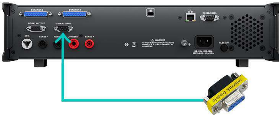
Figure 6-3 Interlock Switch Installation
