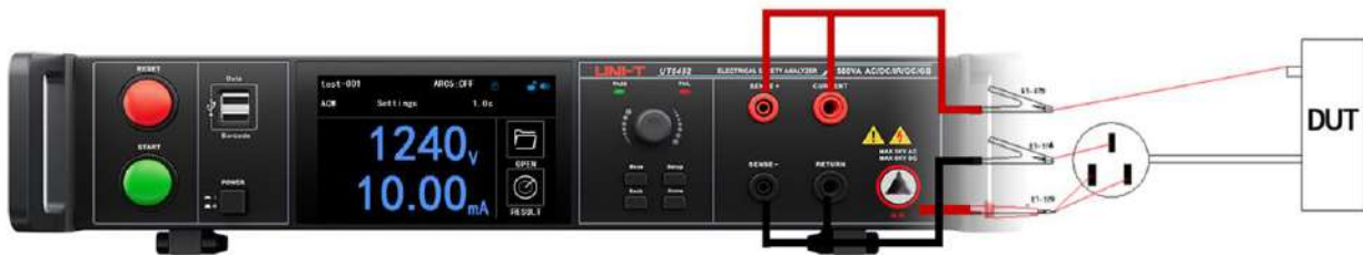
Figure 6-34 Wiring with DUT (UT5430/UT5452)
