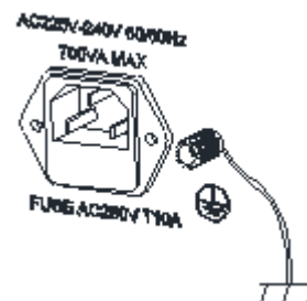
(b) Grounding Via Rear-Panel Ground Terminal
