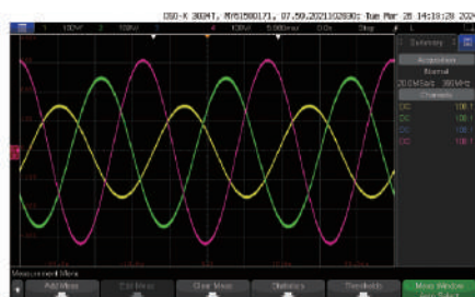
Three-phase unbalanced output (amplitude unbalance + Angle unbalance)
